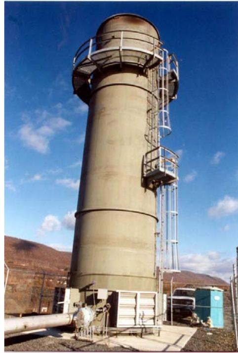
Fig. 4. Typical Enclosed Flare (Courtesy TCE – Ref. 3)
