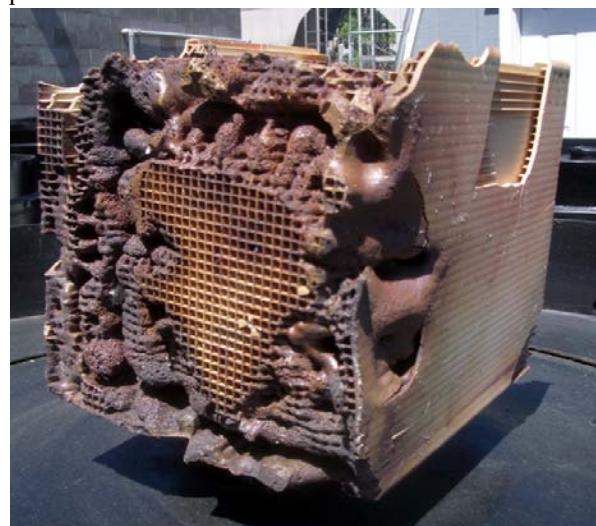
Fig. 9. Damaged RTO packing.
