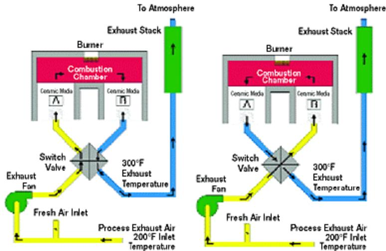
Fig. 6. Typical RTO Operating Diagram (courtesy of MEGTEC Systems – Ref. 5)
