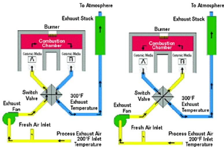
Fig. 6. Typical RTO Operating Diagram (courtesy of MEGTEC Systems – Ref. 5)
