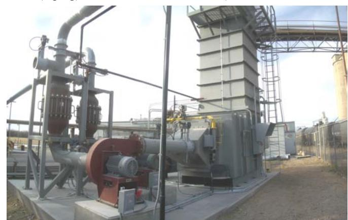
Fig. 11. The DFTO system in operation. Waste air enters the Detonation Arrestors from the top and is transferred to the DFTO burner via the red Process Blowers.
