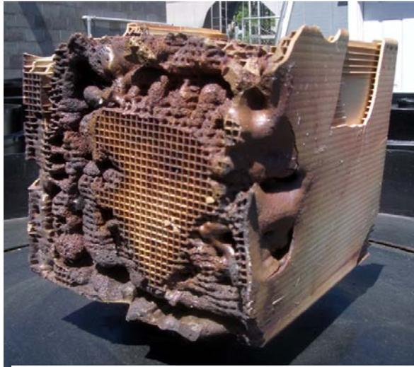
Fig. 9. Damaged RTO packing.
