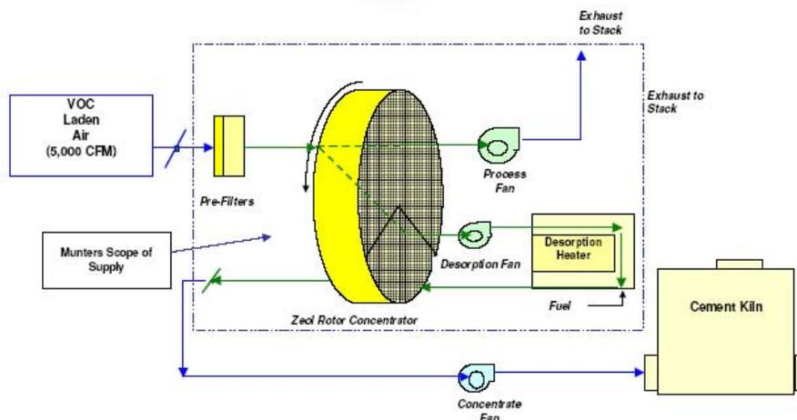
Fig. 5. Diagram shows Munters (Ref. 4) concentrator proposal for Systech vent gas disposal (kiln rather than DFTO)
