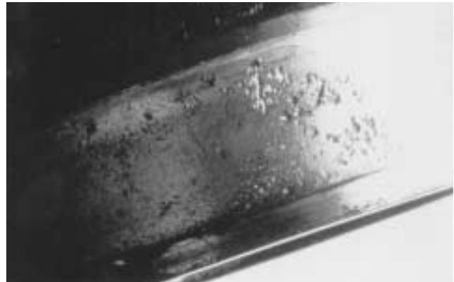
to-metal contact. This can be due to adding an insufficient amount of lubricant when relubricating, too long of a period between relubrications, using dirty lubricant, or using a lubricant that does not have the viscosity needed to maintain an oil film between the parts.
