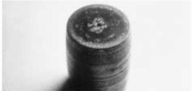
Figure 16. Puddle Corrosion
