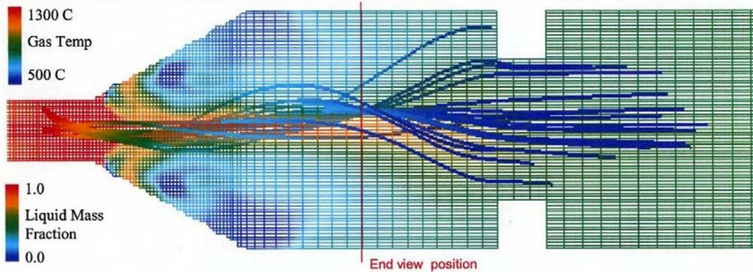
CFD model investigates the evaporation of waste liquid droplets in this waste gas incinerator. The white rectangles are a brick choke ring midway through the furnace. The fuel burner is at left. The exhaust exits to the right into a Watertube boiler, so complete droplet evaporation is needed to avoid tube fouling and emission problems. Note how the choke ring smooths the flue gas temperature variations.
