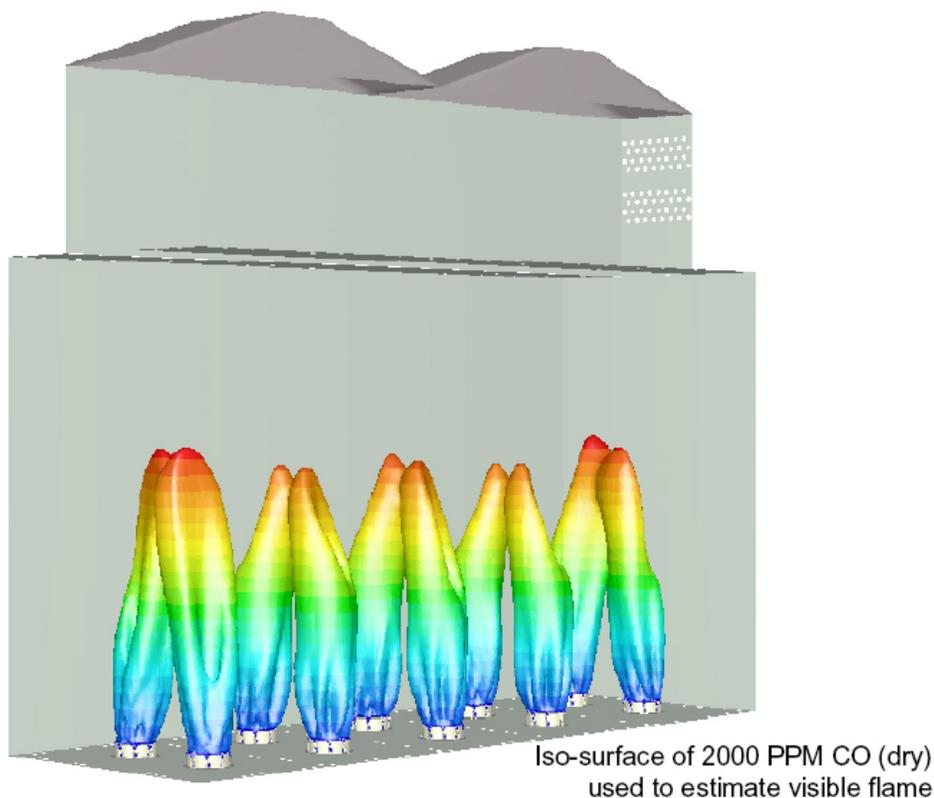
CFD can calculate hydrocarbon destruction – a visible flame contains more than 2000 ppm of carbon monoxide, providing a way to estimate the shape and size of burner flames.
