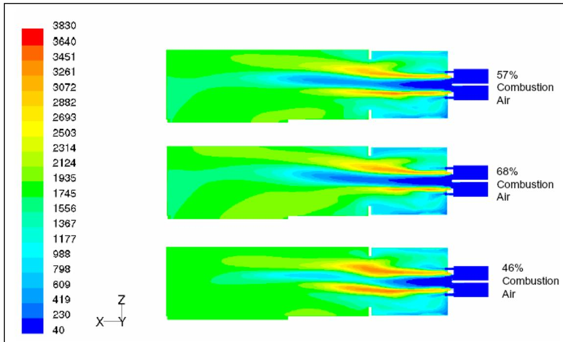
CFD Model of waste gas incinerator showing the effect of varying the amount of combustion air flowing to the burner – 46% air resulted in more even temperature distribution at the furnace exit. Note how the brick choke ring (white bars towards the burner end of the furnace) affects the temperature spread.
